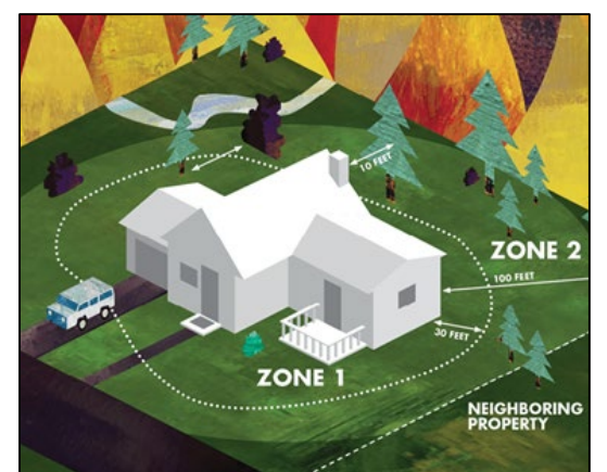
Above is an example of the zoning for creating a defensible space.
